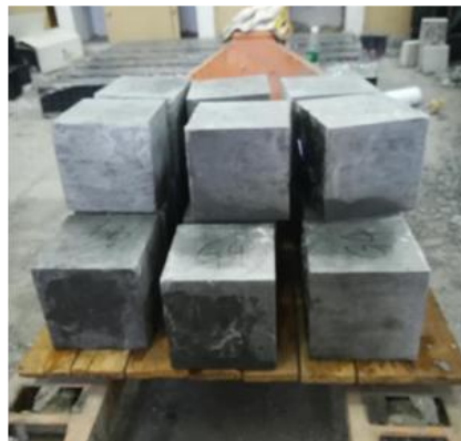
Figure 2. Concrete specimens for the compressive strength test.
