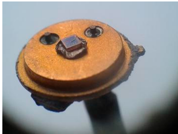
Figure 15. Schottky sensor structure with broken Au wire, after operation in real industrial conditions. Die-pad bonding with Au-In preform (comparison with Figure 2b—bonded with silver nano-paste).
