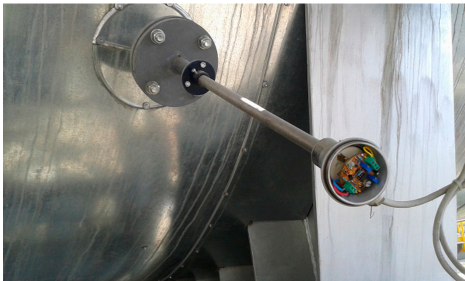
Figure 13. Industrial SiC-Schottky temperature probe mounted at the output of the raw meal mill. Connecting head open in order to reveal read-out circuit mechanical compatibility. D17 as sensing element.
