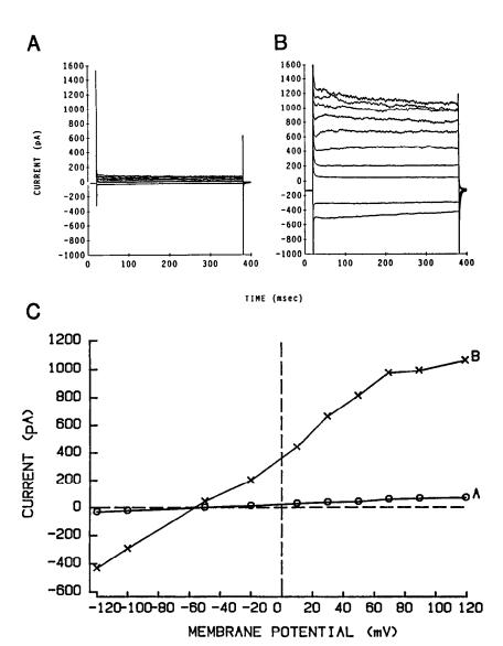
Figure 10. Comparison of currents obtained from 2 separate cells with and without processes. Four out of the seven cells tested that remained without processes after 2 weeks in culture exhibited linear high-resistance membranes. Pulse protocol was as described in Figure 1,  $V_h = -80$  mV. A, Current trace from a cell without processes. B, Current trace from a cell with processes. C, Current-voltage relationship for the 2 cells depicted in A and B.
