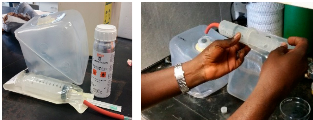
Figure 1. The Detia-Degesch knockdown test kit. The components of the kit (left) are: A collapsible 3.8 L plastic container in which the magnesium phosphide tablet is combined with water to generate about 6000 ppm of phosphine upon reaction; the unopened plastic syringe for use in exposing beetles to gas; and the gas-tight metal container storing the individual sealed tablets of magnesium phosphide. On the right is the transparent plastic syringe with test beetles inside while being loaded with the 6000 ppm phosphine prior to drawing in an equal volume of fresh air to dilute the chamber concentration to about 3000 ppm.
