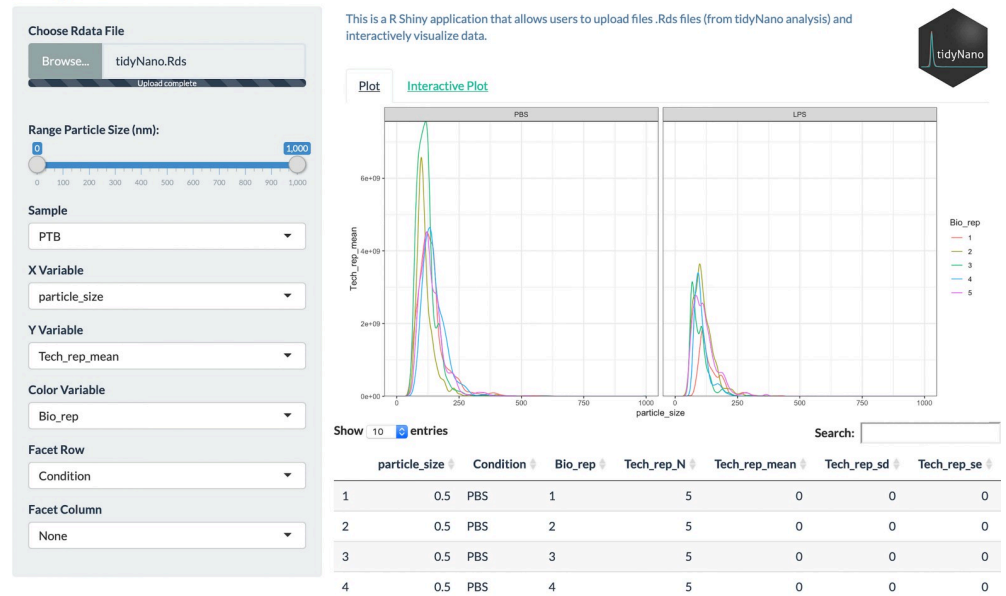
Fig 5. Interactive data manipulation and visualization with shinySIGHT web application. shinySIGHT allows users to upload tidyNano data to visualize and manipulate data using a graphical user interface. shinySIGHT automatically generates plots from user uploaded data as well as displays the underlying data frames that make up the visualizations.
