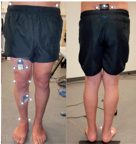
Figure 4. Sensor and marker placement for the single leg squat experiment in the Motion Capture Lab.
