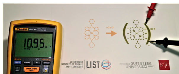
Figure 2. Optical image of the sublimed NiDPP coating (orange, left) and patterned oCVD NiDPP coating (green, right) deposited on paper. The green oCVD NiDPP coating displays electrical conductivity.
