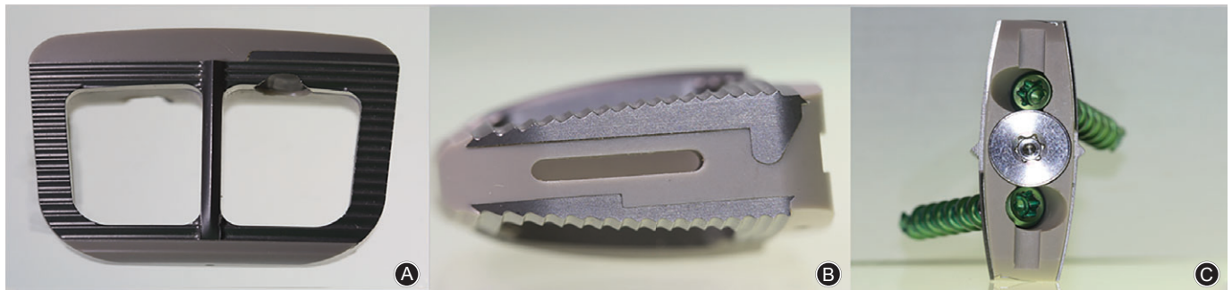
Fig. 5 Redmond lumbar cage (A-SPINE Asia). (A) Superior view showing central beveled keel. (B) Lateral view showing angulated ridges and composite design and Ti end-plate inlay, fixed in a PEEK body. (C) Anterior view showing two integrated screw fixation.
