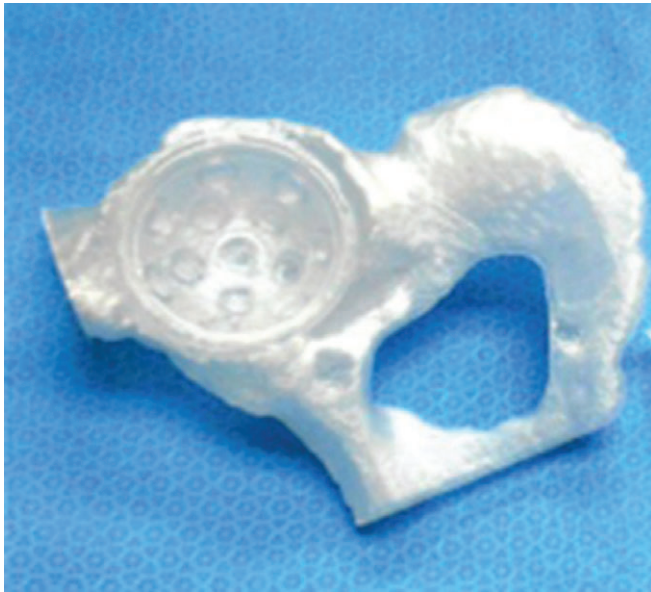
Fig. 8 A 3D printed patient-specific implant (PSI) right acetabular cup placed in a native acetabulum/pelvis patient-specific model. Both the model and implant were manufactured based on a patient computed tomography (CT) scan, and were printed with an SLA 5000 3D printer from 3D systems using Watershed XC11122 resin 42 .
