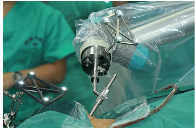
Fig. 4 A cannula is inserted through the robotic sleeve to reach the bone cortex, after which a K-wire is placed through the cannula.
