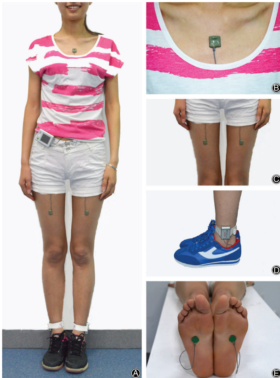
Fig. 1 Intelligent Device for Energy Expenditure and Activity (IDEEA) system: (A) composition of IDEEA; (B) the sensor on chest; (C) the sensors on thighs; (D) the sensors on ankles; and (E) the sensors on the bottom of feet.
