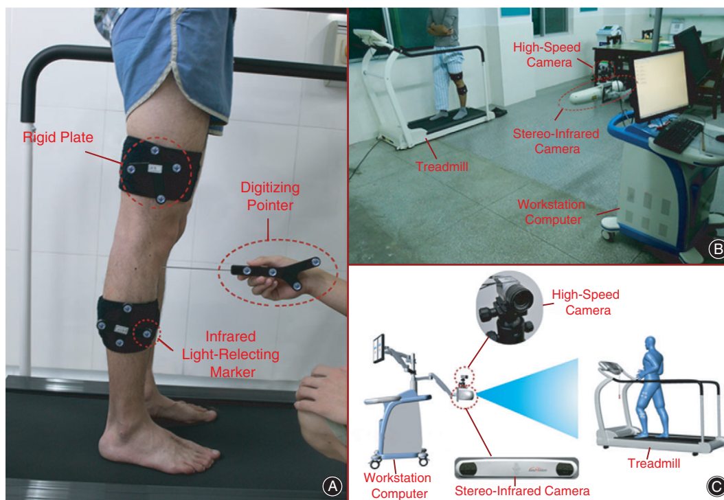
Fig. 2 (A) Identification of surface markers. Two rigid plates, each composed of four infrared light-reflecting markers, are attached to each subject's thighs and shanks with bandages. A digitizing pointer composed of four infrared light-reflecting markers is used to identify femoral and tibial landmarks. (B) The instrument for knee kinematics analysis. The 3-D trajectories of the rigid plates during activities are tracked by an integrated two-head stereo-infrared camera at a frequency of 60 Hz. An integrated synchronous high-speed camera is used to divide the walking cycle and to record video of the activity. A workstation computer with customized software performs supplementary real-time calculations. The entire system is integrated on a mobile cart (1.1 m × 0.6 m × 0.4 m). Each subject was asked to walk on a horizontal treadmill at a speed of 3 km/h. (C) Schematic representation of the instrument for knee kinematics analysis.
