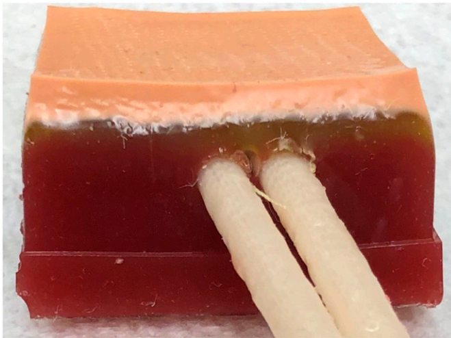
Figure 2. The vascular access pad is a three-layer model. The tan tone at the top of the picture is 2–3 mm deep. The epidermis is 2–3 mm thick with yellow coloring to simulate fat. The hypodermis extends beyond a depth of 1 cm with vessels imbedded in the red polymer.
