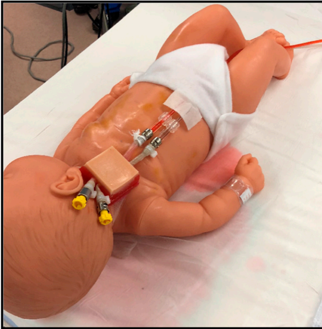
Figure 5. The surgical pad is secured using extra mesh that was imbedded with the epidermis layer. Metal male luer connectors are used with either tape or Panduit tie bands on both sides of the blood vessels. Priming with either the static or Calafia model is simplified by removing the male cap distal to the vessel.
