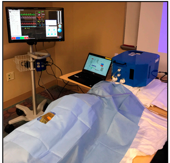
Figure 7. The Calafia simulator is attached using standard connectors with the unit slightly higher than the level of the venous vessel. This height, like the static Buretrol model, mimics the mean venous pressure. Activating the pulsatile mode with the Calafia, the arterial mean pressure and pulsation mimic the arterial vessel.
