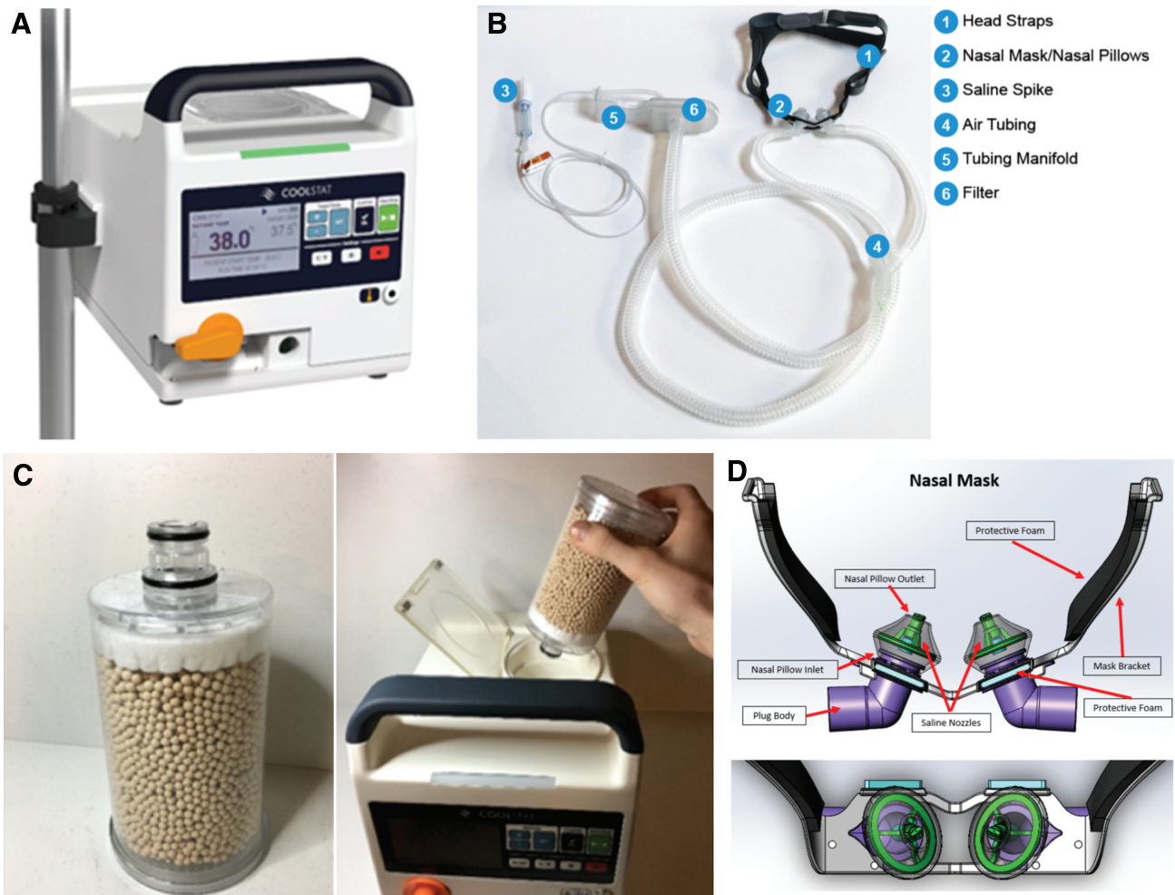
FIG. 3. Transnasal cooling therapy system. (A) CoolStat device. (B) Nasal mask and plastic tube set (disposable). (C) CoolStat™ disposable desiccant cartridge and loading in device. (D) Nasal mask in detail. Saline nozzles are placed inside the nasal pillows, throughout which small amounts of saline are periodically misted into the nostrils. Color images are available online.
