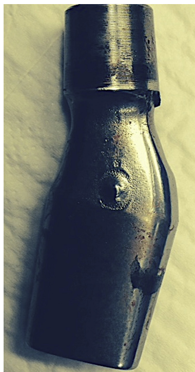
Figure 3. Intraoperative image of Zimmer Kinectiv titanium modular neck demonstrating corrosion product at head-neck and neck-stem junctions.
