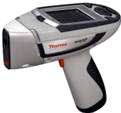
Fig. 2. PMI testing equipment to evaluate the elemental analysis of dental implants.
