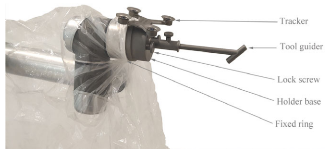
Fig. 3 TianJi Robot navigation and positioning tool installation, including fixed ring, tracker, tool guider, lock screw, and holder base.
