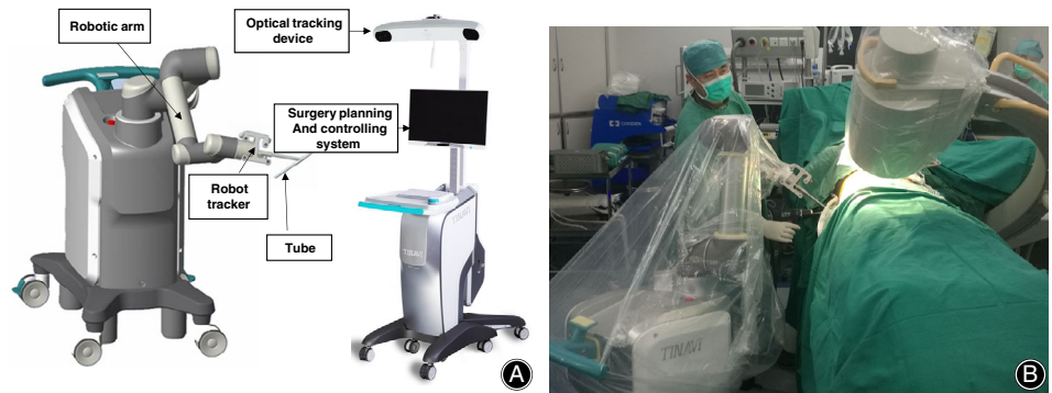
Fig. 1 The bi-planar robot navigation system construction (A) includes a robotic arm, an optical tracking device, and a surgery planning and controlling system. (B) The robot arm provided a guide channel for the surgeon during the operation.
