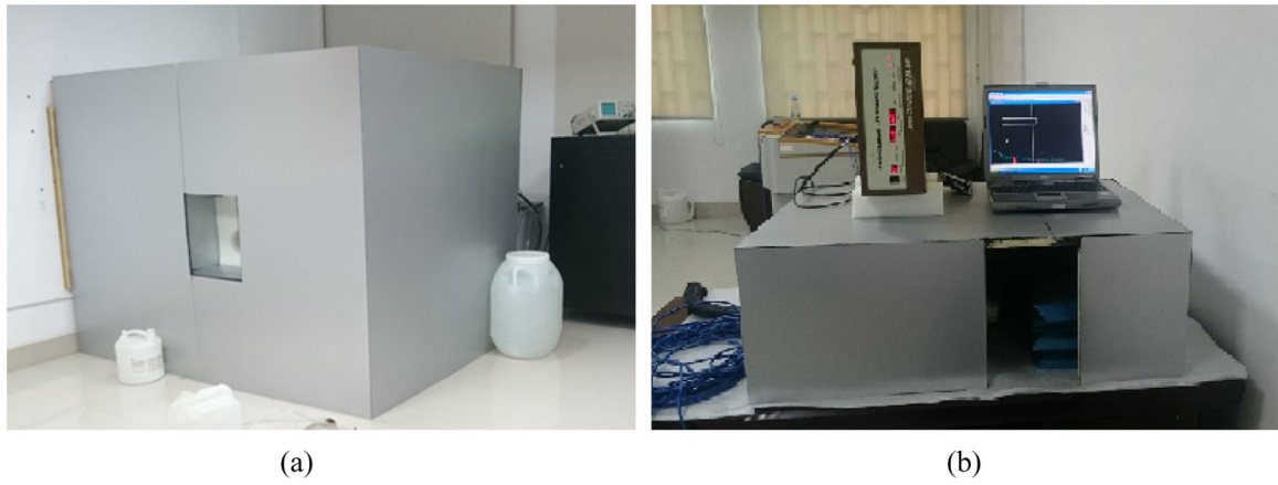
Figure 1. The neutron irradiation system (a) and the HPGe \gamma -ray measurement system (b).
