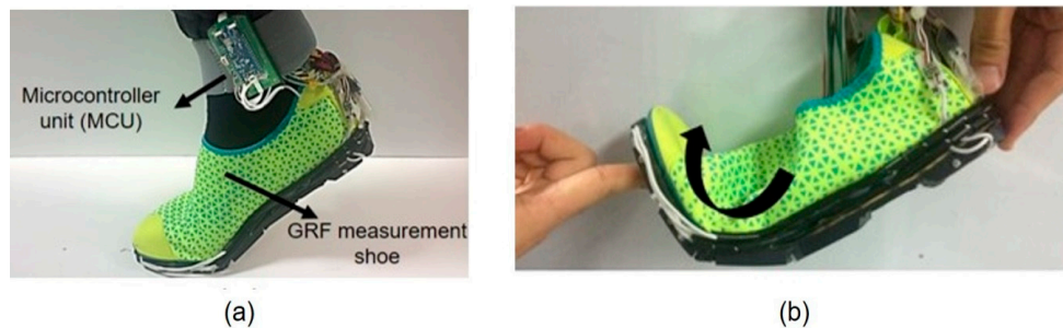
Figure 2. Bendable outsole biaxial ground reaction force measurement system. (a) Developed system connected to the microcontroller with a Bluetooth module. (b) Developed system with a bendable design.
