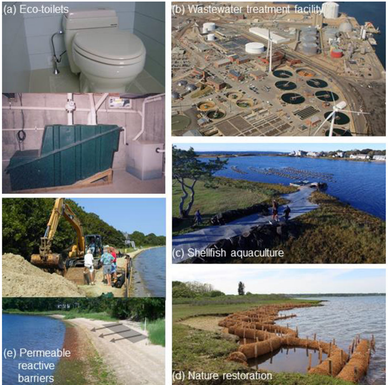
Fig. 4. The effectiveness of strategies to reduce anthropogenic nitrogen inputs in coastal water bodies is being evaluated on Cape Cod. (a) Urine-diverting and composting eco-toilets (top panel) are options for individual homes, businesses, or public areas. The waste collection system (bottom panel) uses gravity to separate urine from solids for nitrogen removal. (b) Wastewater treatment facilities provide industrial scale means to remove nitrogen from human waste. (c) Commercial aquaculture of oysters, clams, and mussels is a cultural heritage on Cape Cod. More recently, the practice is considered to be an option to denitrify
