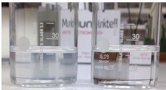
Figure 3. Feed (left) and permeate (right) in filtrations of SWW through nanocellulose filter papers. The total solid content of the feed dispersion was 0.251 \text{ mg L}^{-1} .
