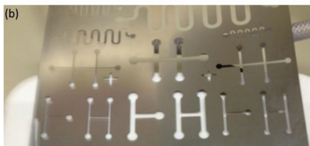
Figure 4. a) Design of microfluidic channels. Photos of b) PDMS mask and c) deposited CNF pattern on PET. d) Simplified schematic view of the microfluidic channel which is formed between CNF patterns in the assembled device.
