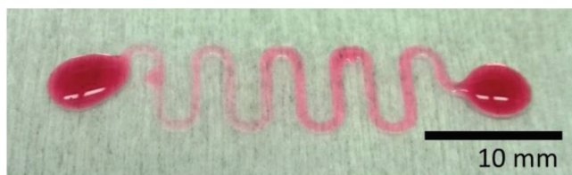
Figure 3. Colored water deposited on spray-coated CNF pattern on a PET substrate.
