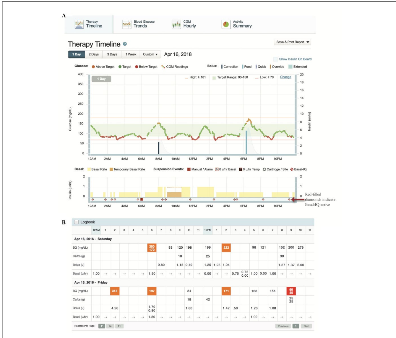
Figure 12. Therapy Timeline Report. (A) Therapy detail. Types of bolus and basal are displayed as colored bars on this report: Food Bolus (light blue bar), Correction Bolus (dark blue bar), Basal (yellow area), Temporary Basal (orange area). (B) Log Book. Data including date and time, BG, carb amount, and insulin delivery.
