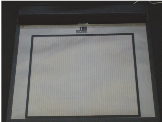
FIGURE 1: The postural platform (MatScan, Tekscan Inc., Boston, MA, USA) used for the purposes of this study.
