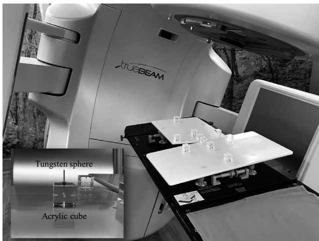
FIG. 4. Photograph of the cubic phantoms installed to confirm the rotational accuracy of the prototype device by Varian cone-beam computed tomography imaging system. The tungsten sphere of 1 mm at diameter was inserted into each acrylic cube
