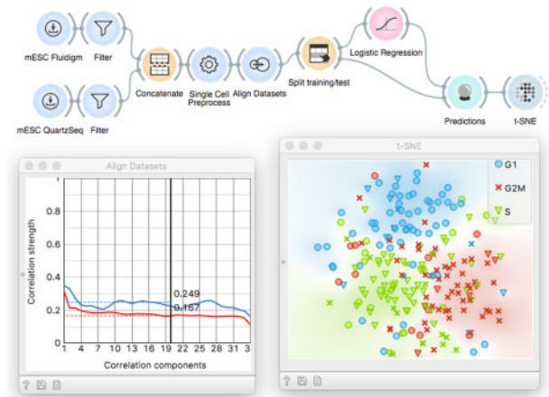
Fig. 10. Workflow that showcases the inference and utility of cell classification model. Here, we predict cell cycle phase by learning a model on one dataset and applying it on another one. Gene expressions are made comparable with Align Datasets . A logistic regression model is trained on the mESC Fluidigm dataset (Buettner et al. , 2015) and the cell cycle phase is predicted for mESC Quartz-Seq (Sasagawa et al. , 2013). The predicted values (colors) almost exactly match the ground truth (symbols) in the t-SNE plot
