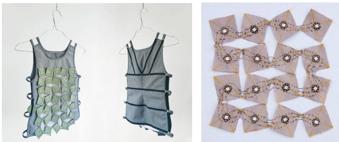
Figure 5. First prototype of the Wearable Breathing Trainer (WBT) with the square-shaped robotic textile and the LED-matrix.
