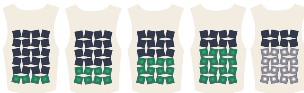
Figure 4. The LED-matrix showing an increase in the lighted rows that indicate the feedback on performance regarding the position of the breath. The white light informs the child that the rhythm was not good.
