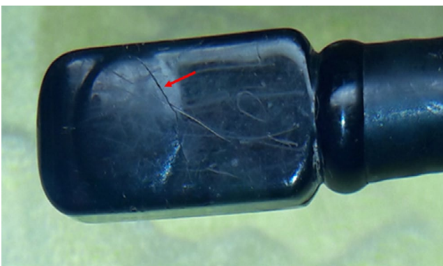
FIGURE 1 The tip of one of the transesophageal echocardiography probes in use during the study period. With magnification and specific lighting used in this photograph, numerous superficial scratches and a crack (arrow) in the plastic casing can be visualized. The damage was not obvious to the naked eye. The outbreak strains of Pseudomonas aeruginosa and Enterococcus faecalis were isolated from this crack, after the probe had been decontaminated and was ready for use (Photo: Thorkell Thorkelsson) [Colour figure can be viewed at wileyonlinelibrary.com ]
