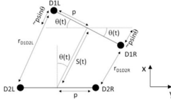
From this construction, we can see that good approximations to the distance between D1R and D2R ( $r_{D1D2R}$ ) and D1L and D2L ( $r_{D1D2L}$ ) are simply:
