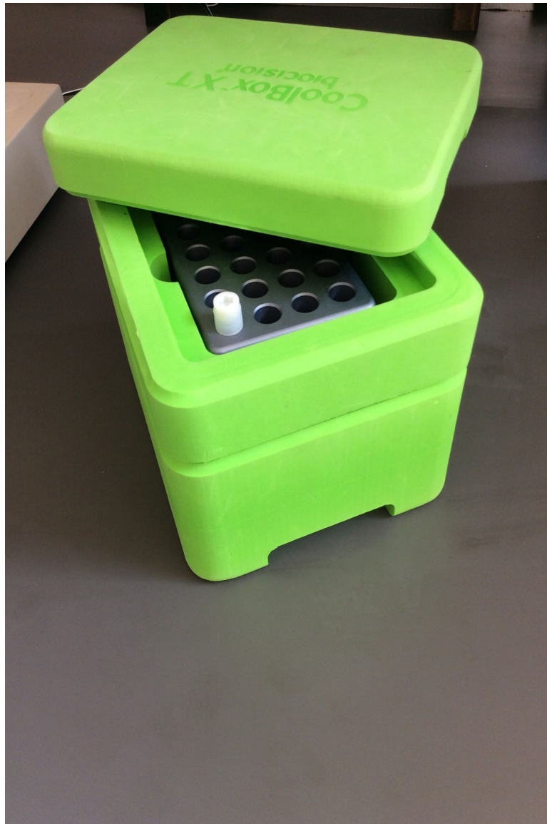
Figure 2. An illustration of a sample stored in portable freezing storage container (BioCision CoolBox XT CryoTube 24 Workstation, BioCision Catalogue No. BSC-575).
