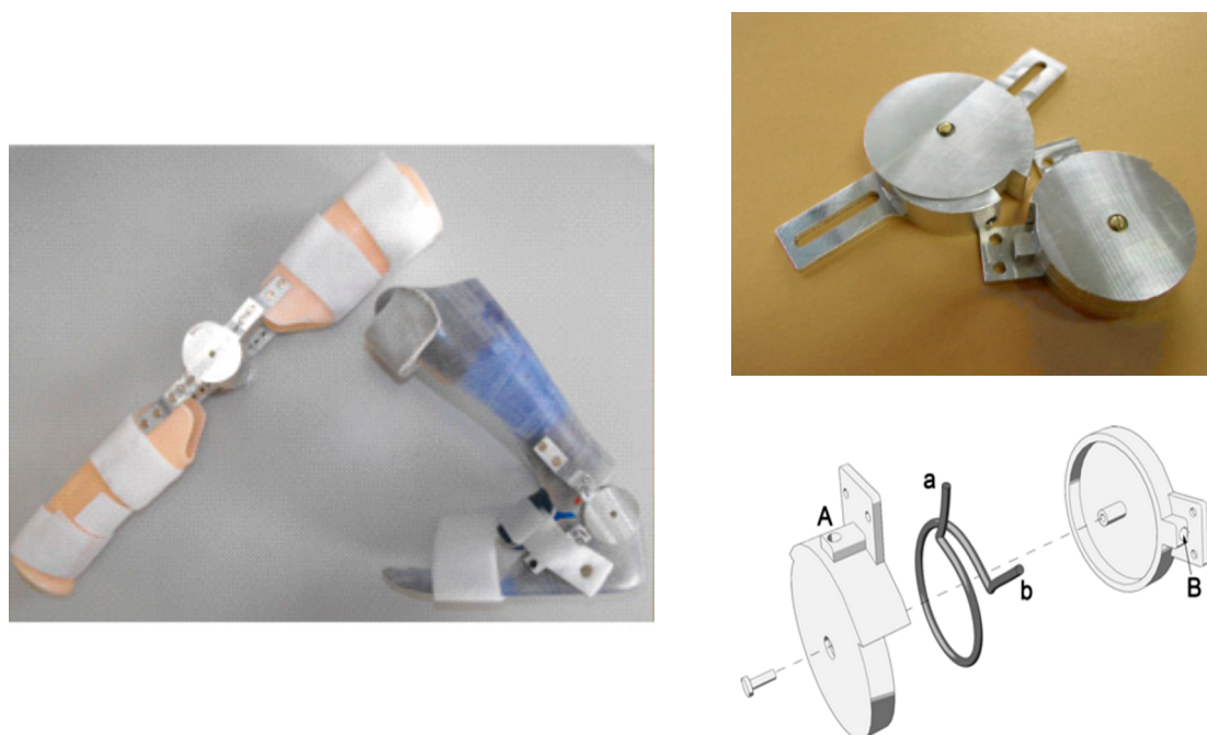
Figure 11. The pseudoelastic hinges consist of two parts rotating around a common central axis. Within the inner chamber formed by the two parts, a pseudoelastic \Omega -shaped spring is inserted which generates a torque between two half-hinges. The ends (a and b) of the pre-loaded spring are inserted into the corresponding holes (A and B, respectively) in the parts [32,33].
