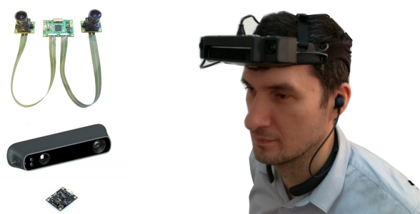
Figure 1. The Sound of Vision headgear: (left) 3D acquisition devices integrated in the SoV system—stereo camera (LI-OV580 from Leopard Imaging), IR depth sensor (Structure Sensor PS1080 from Occipital), IMU device (LPMS-CURS2 from Lp-Research) and a prototype implementation of the SoV headgear (right).
