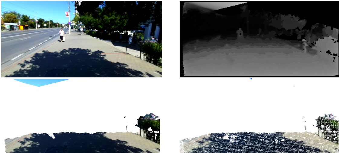
Figure 3. Comparison between our reconstruction and single frame based reconstruction. (Top-left) RGB image from the left camera. (Top-right) Disparity map computed with the approach of [33]. (Bottom-left) 3D reconstruction constrained within 5 m in front of the camera, based solely on the disparity map of the current frame. Errors in the estimation of the stereo correspondence lead to the presence of false structures in the reconstruction. (Bottom-right) Result of our incremental reconstruction showing the accumulated stable points (confidence above a predefined threshold).
