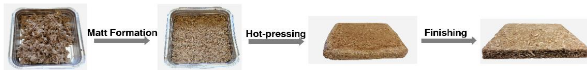
Figure 1. Steps of manufacture process of particleboards bonded with a sour cassava starch, starting with a mixture of wood particles and starch paste and ending with a finished particleboard.
