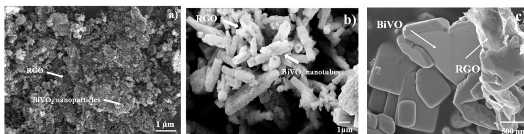
Figure 1. SEM images of \text{BiVO}_4 / reduced graphene oxide (RGO): (a) \text{BiVO}_4 nanoparticles/RGO; (b) \text{BiVO}_4 nanotubes/RGO; (c) \text{BiVO}_4 nanosheets/RGO.
