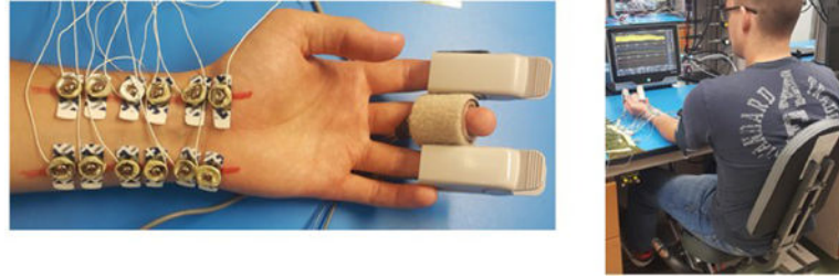
Fig. 4. Pictures showing the placement of electrodes and sensors on the wrist and fingers (left) and the experimental setup for BP monitoring (right).
