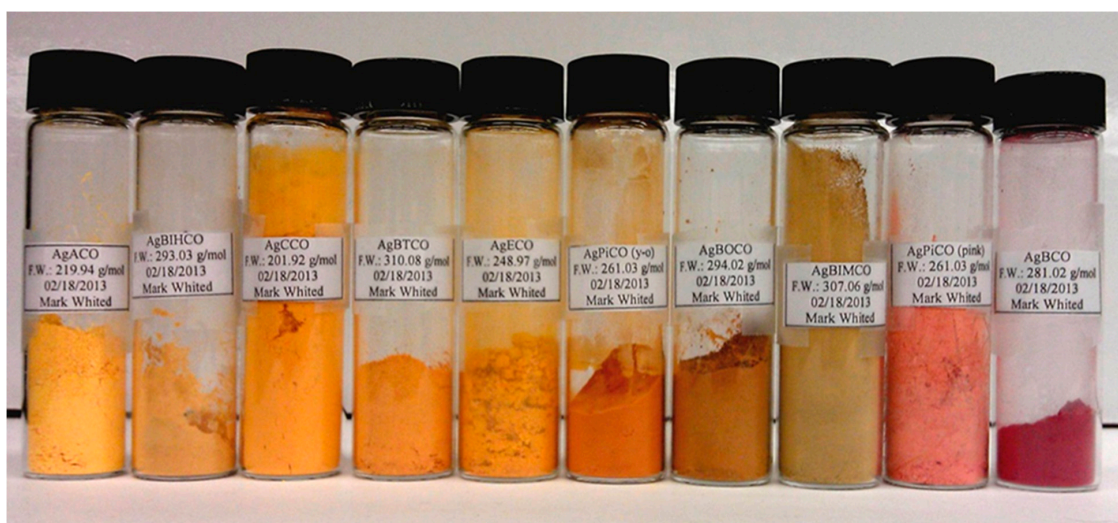
Figure 1. Pyrex vials with visible light insensitive, thermally stable, sparingly water soluble and antimicrobial Silver(I) cyanoximates: demonstration of variety of unusually bright colors of complexes.
