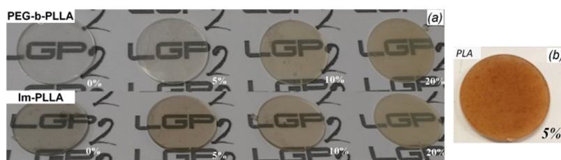
Figure 2. Disks prepared by injection-molding of extruded samples of (a) PLA and the surfactant (the value on the right side of the disk is related to the CNC content) and (b) PLA and 5 wt % uncompatibilized CNCs.
