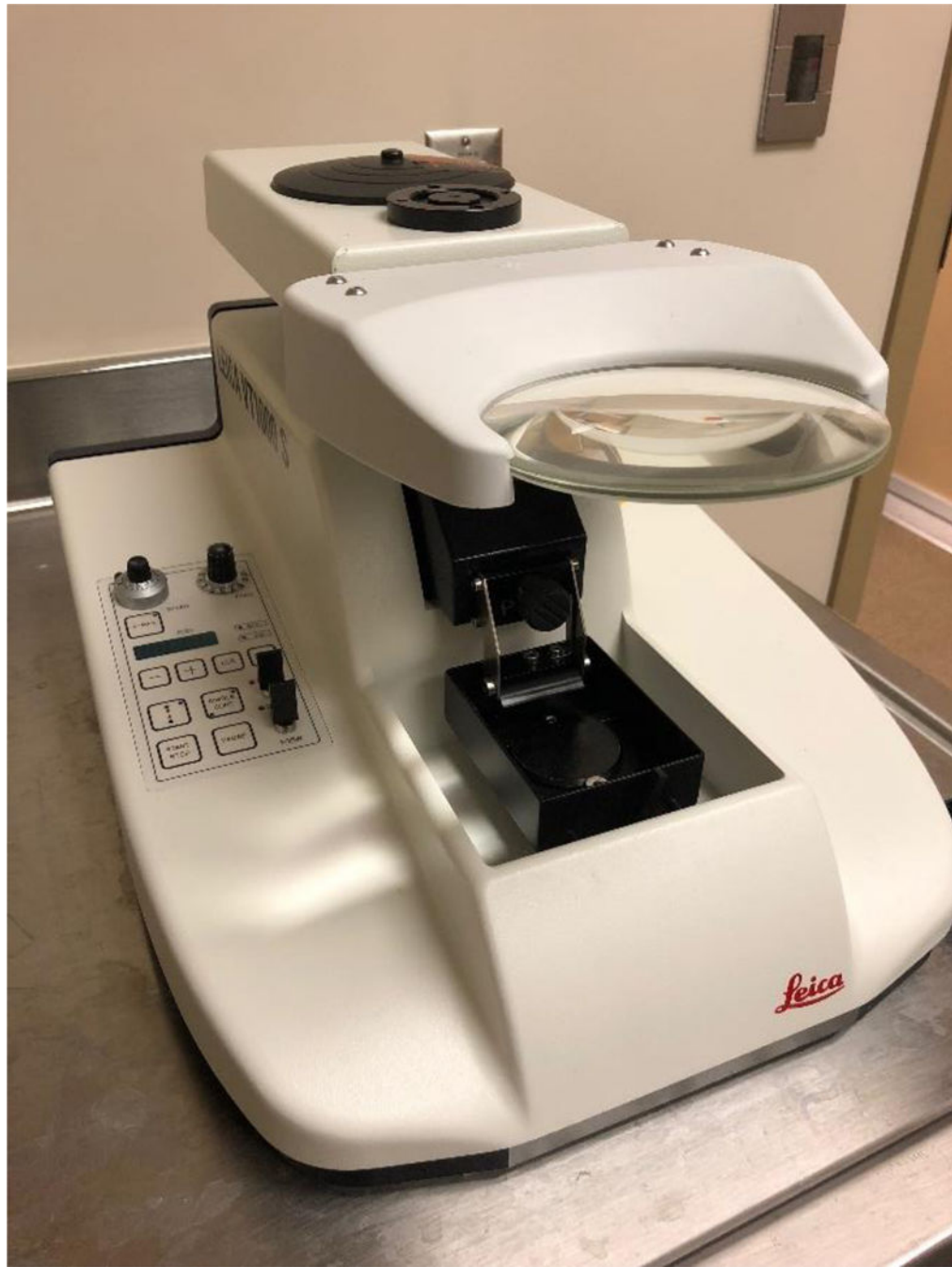
Figure 4: A commonly used motorized, oscillating tissue microtome (vibratome) used for preparing thin (between 100–300 \mu\text{m} thick) tissue slices for electrophysiology (Leica Microsystems, Wetzlar, Germany).
