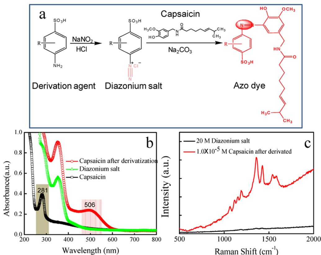
Figure 1. Derivatization reaction route of capsaicin (a). UV-vis spectra (b) and SERRS spectra (c) of capsaicin and its derivation agent.
