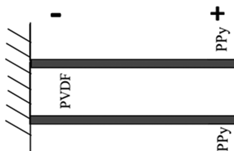
Figure 4. Equivalent model of PPy trilayer actuator.
