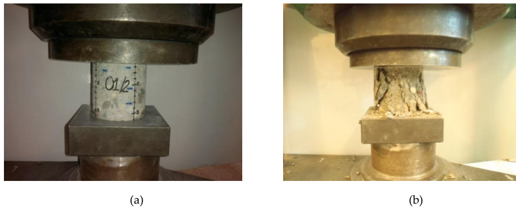
Figure 9. The sample in strength testing machine: (a) during loading, (b) after failure.
