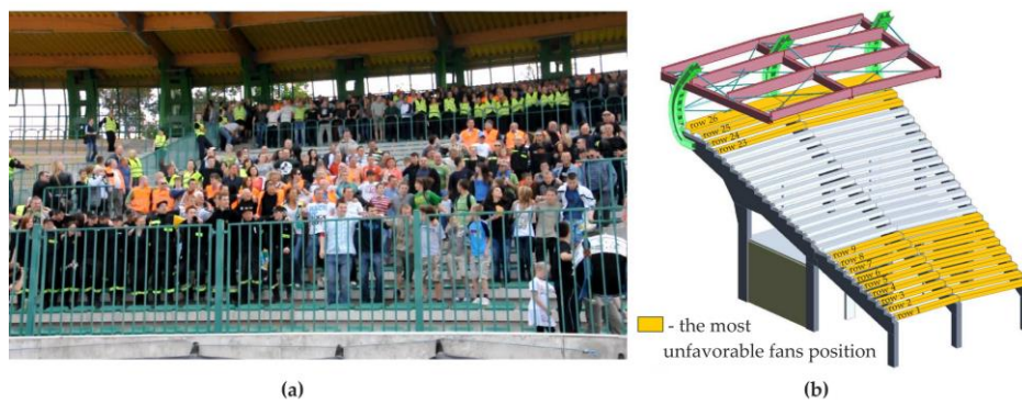
Figure 8. Dynamic tests with fans: (a) experimental setup, (b) scheme showing the arrangement of people during tests (orange color—rows indicating the most unfavorable fan positions).
