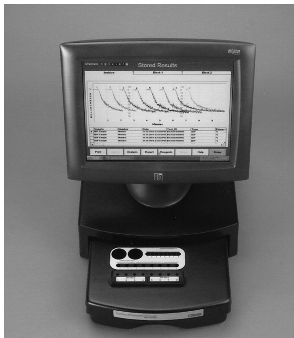
Figure 1: Turbidometric platelet aggregometer. It measures the decrease in light transmittance that results from platelet coaggregation in platelet-rich plasma, when samples are exposed to an agonist such as ADP. Reproduced with permission from Harrison P et al. 5
