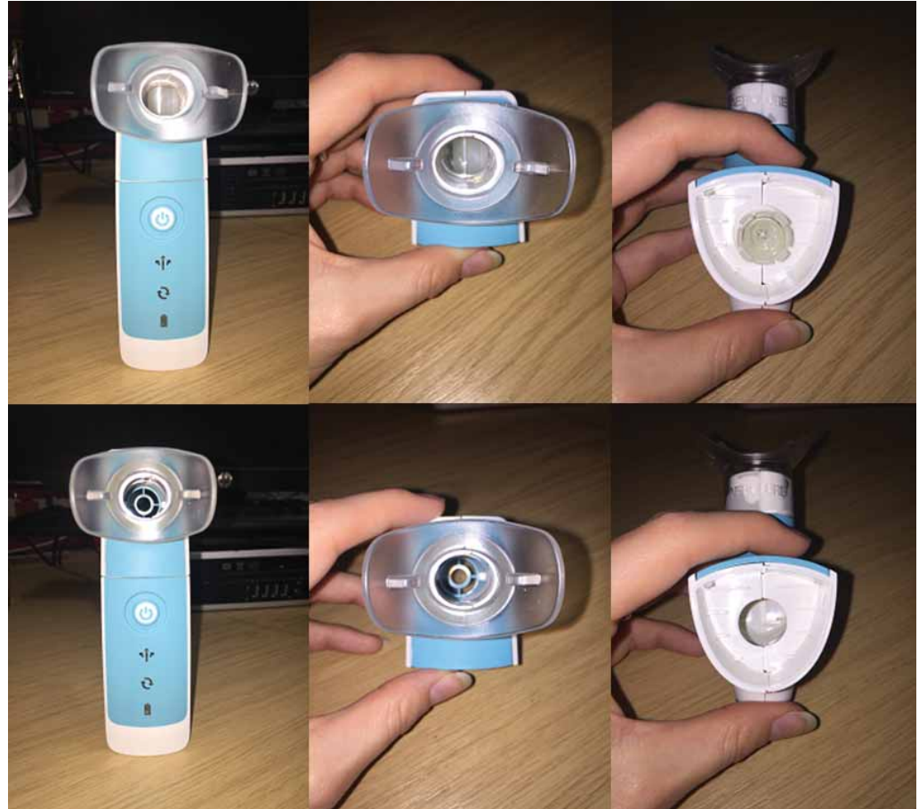
FIGURE 2 Top (left to right): Aerosure Medic active device, and device aerosol head anterior and inferior views. Bottom (left to right): Aerosure Medic sham device, and device aerosol head anterior and inferior views. Note mechanism removed from sham device.
