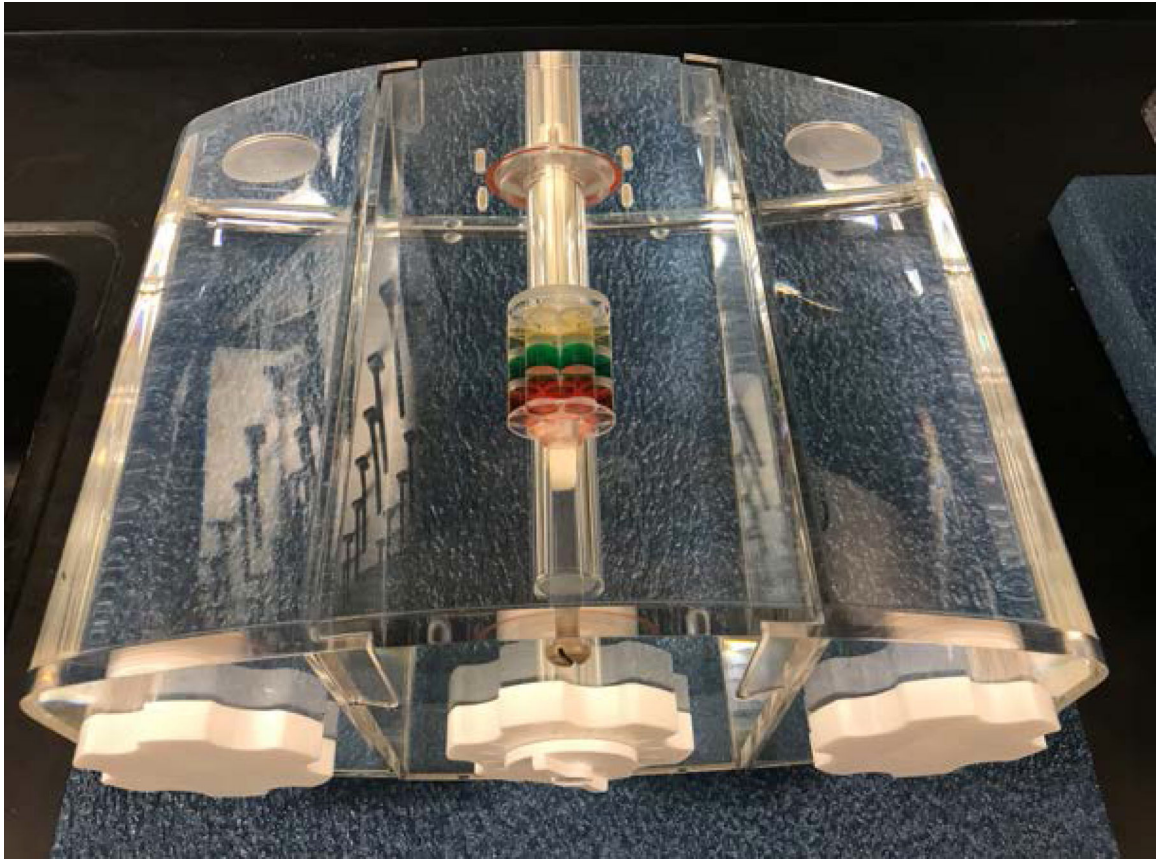
Figure 1: Top-view of the UMN/HPD anthropomorphic, prostate, body-imaging reference object. This three-sectioned body phantom has a quantitative prostate mimic at its center (i.e. yellow, green and red structure) and can accommodate surface and endorectal coil configurations.
