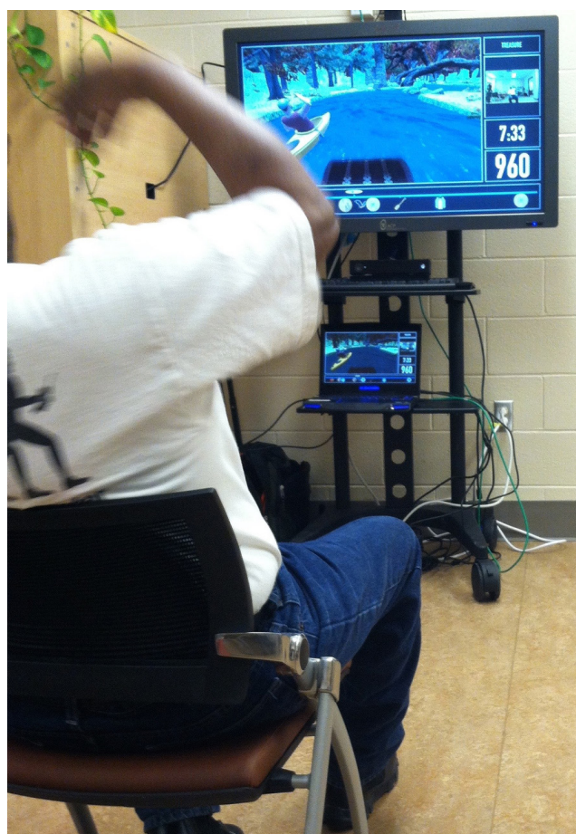
Figure 1. In Recovery Rapids, movements of the participants' more affected upper extremity, captured via the Xbox 360 Kinect sensor, drive game play. The participant's posture and reaching action are reflected in the avatar's position.
