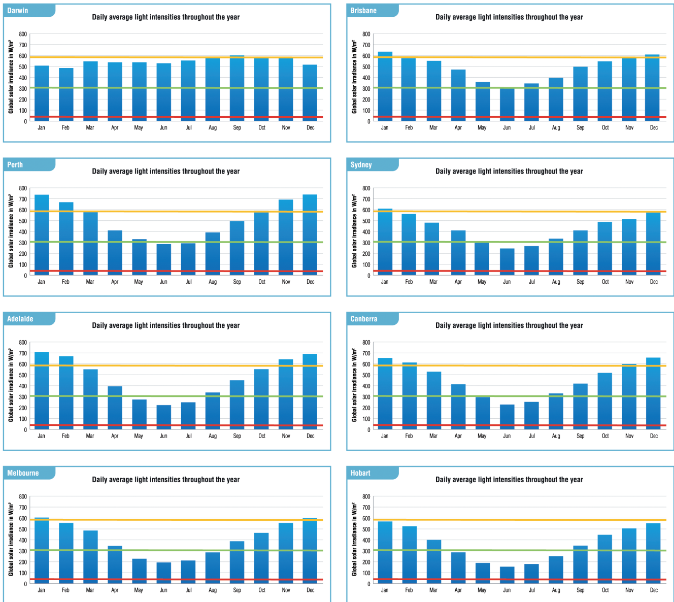
Figure 2 Modelled daily average global radiation for each month (Meteonorm data 1986–2005). Horizontal lines indicate light intensity levels of Australian DL-PDT study 12 (red: min. 40 W/m 2 ; orange: max. 585 W/m 2 ; green: average 305.8 W/m 2 ).
