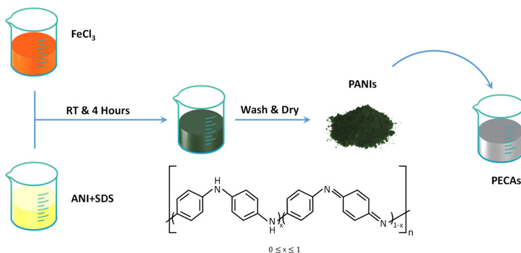
Scheme 1. Illustration of the synthesis of polyanilines (PANIs) by chemical oxidation polymerization process and fabrication of PANIs-enhanced electrically conductive adhesives (PECAs) with excellent electrical property.
