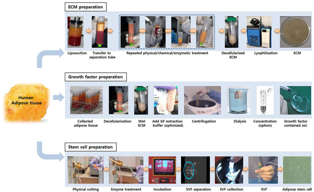
Fig. 1 Scheme for preparation of human adipose tissue-derived extracellular matrix (ECM), growth factors (GFs), and stem cells. Human adipose-derived ECM is collected from liposuction, decellularized, and then manufactured to the required form. The GFs are
